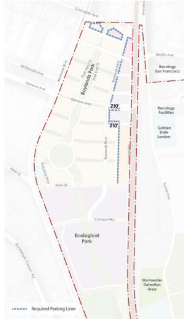
FIGURE 3.2.5 REQUIRED PARKING LINER EDGES
