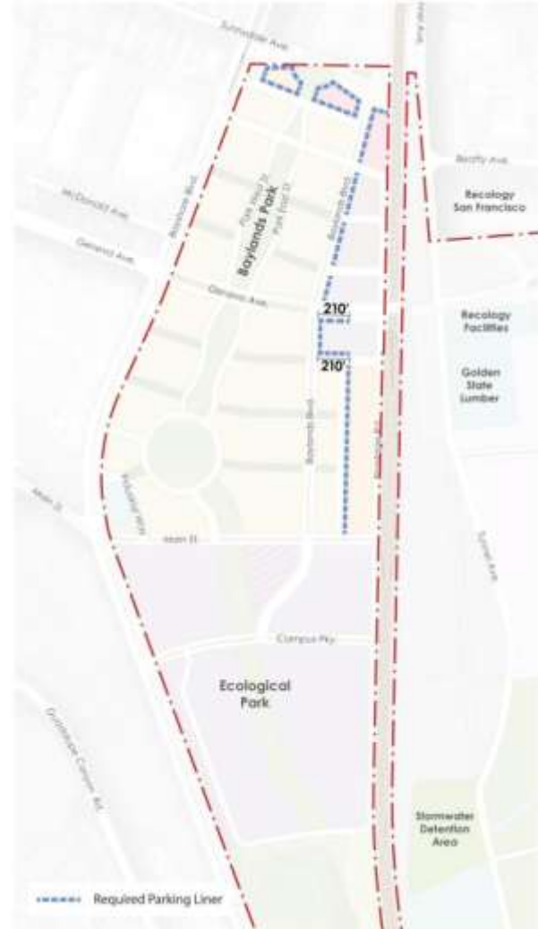
FIGURE 3.2.5 REQUIRED PARKING LINER EDGES
