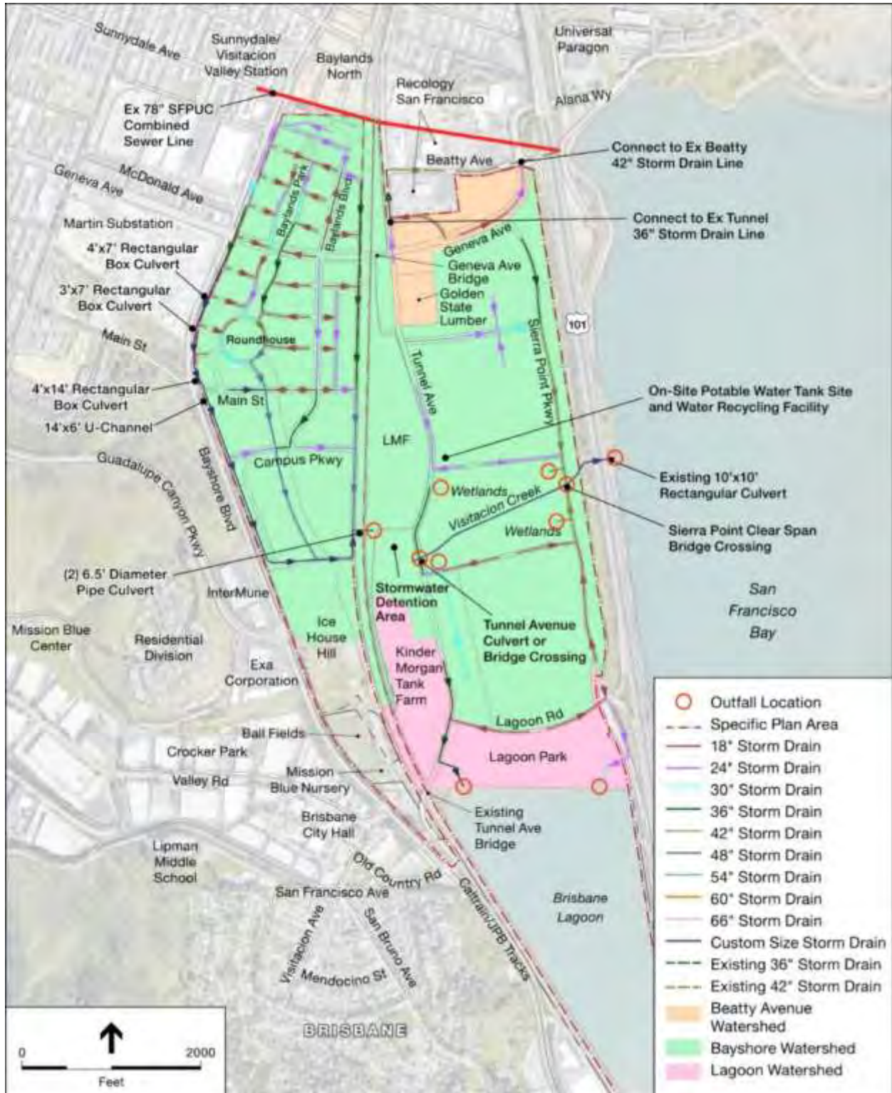
FIGURE 7.4.2. CONCEPTUAL STORM DRAINAGE SYSTEM IMPROVEMENTS
