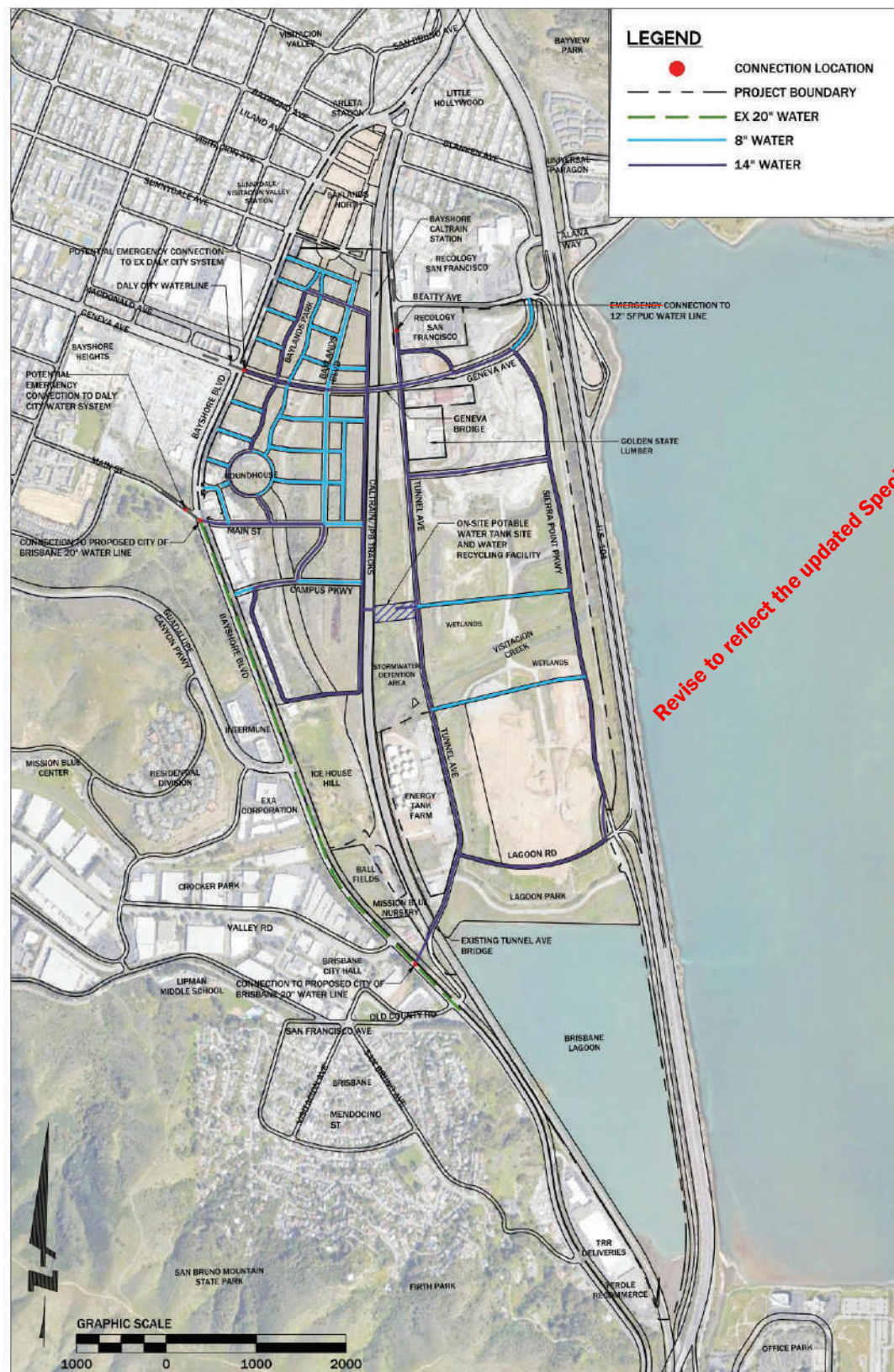
FIGURE 7.3 PROPOSED PORTABLE WATER SYSTEM IMPROVEMENTS
