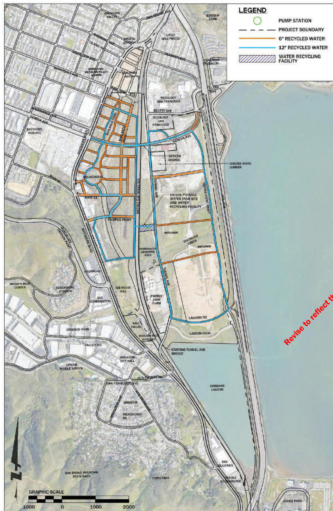
FIGURE 7.4 PROPOSED RECYCLED WATER SYSTEM IMPROVEMENTS
