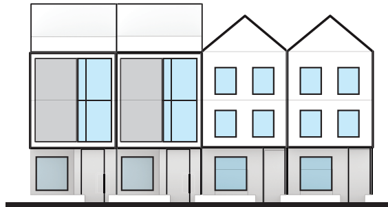
FIGURE 3.51: ELEVATIONS WITH MINIMUM 30% FENESTRATION AREA
