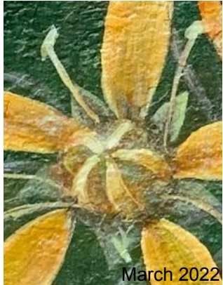
Few examples of flaking paint lifting away from the substrate
